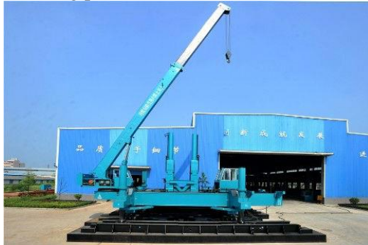
Gambar 2. 1 Hydraulic Pile Injection
