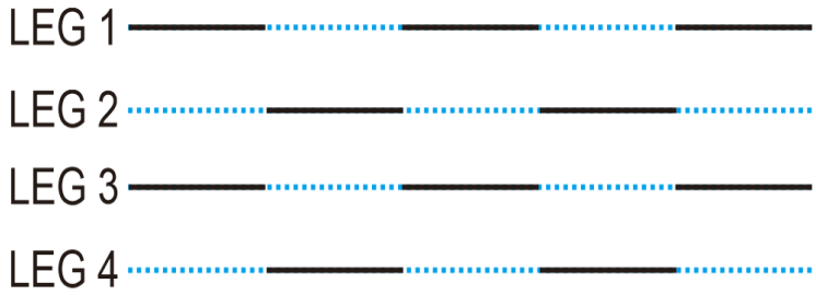
Gambar 3. 24 Diagram Dualpod Gait
