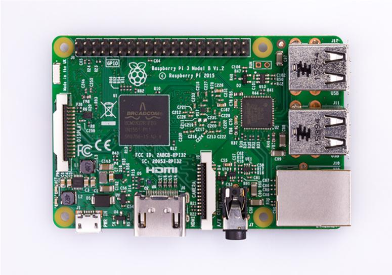
**Gambar 2.2:** Raspberry Pi 3 Model B[12]
