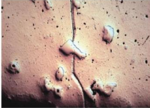
Photomicrograph of Colmonoy 6 fused coating, original at 50x
