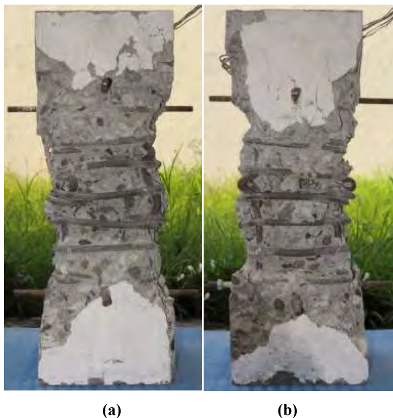
Figure B-13 Specimen CS03a: (a) side 3; and (b) side 4 after the completion of the test
