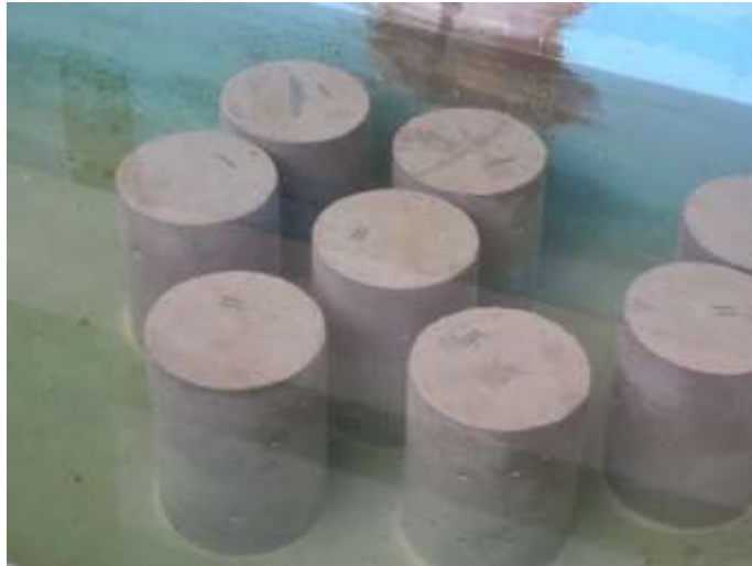
Figure 3-39 Curing of standard cylinders
