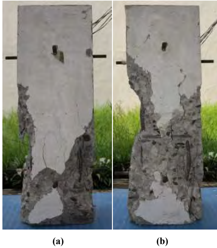
Figure B-9 Specimen CS02a: (a) side 3; and (b) side 4 after the completion of the test
