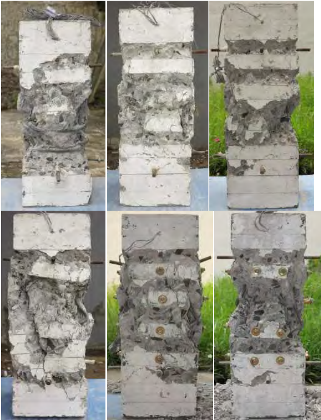
Figure 4-11 Specimens S04a, S04b, S04c, S04d, S04e, and S04f after completion of the tests
