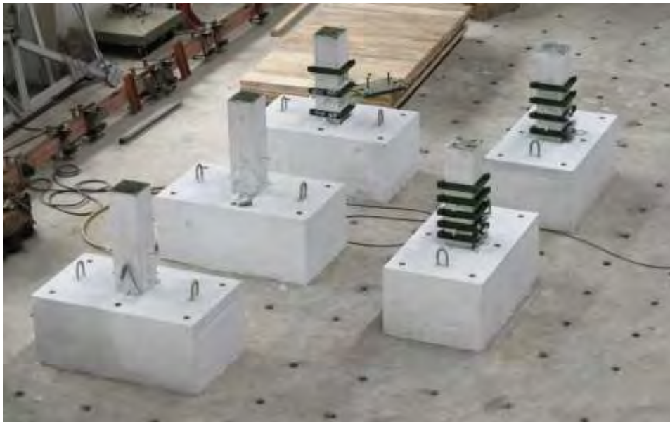
Figure 3-50 The five column specimens for quasi-static combined axial and cyclic lateral load test
