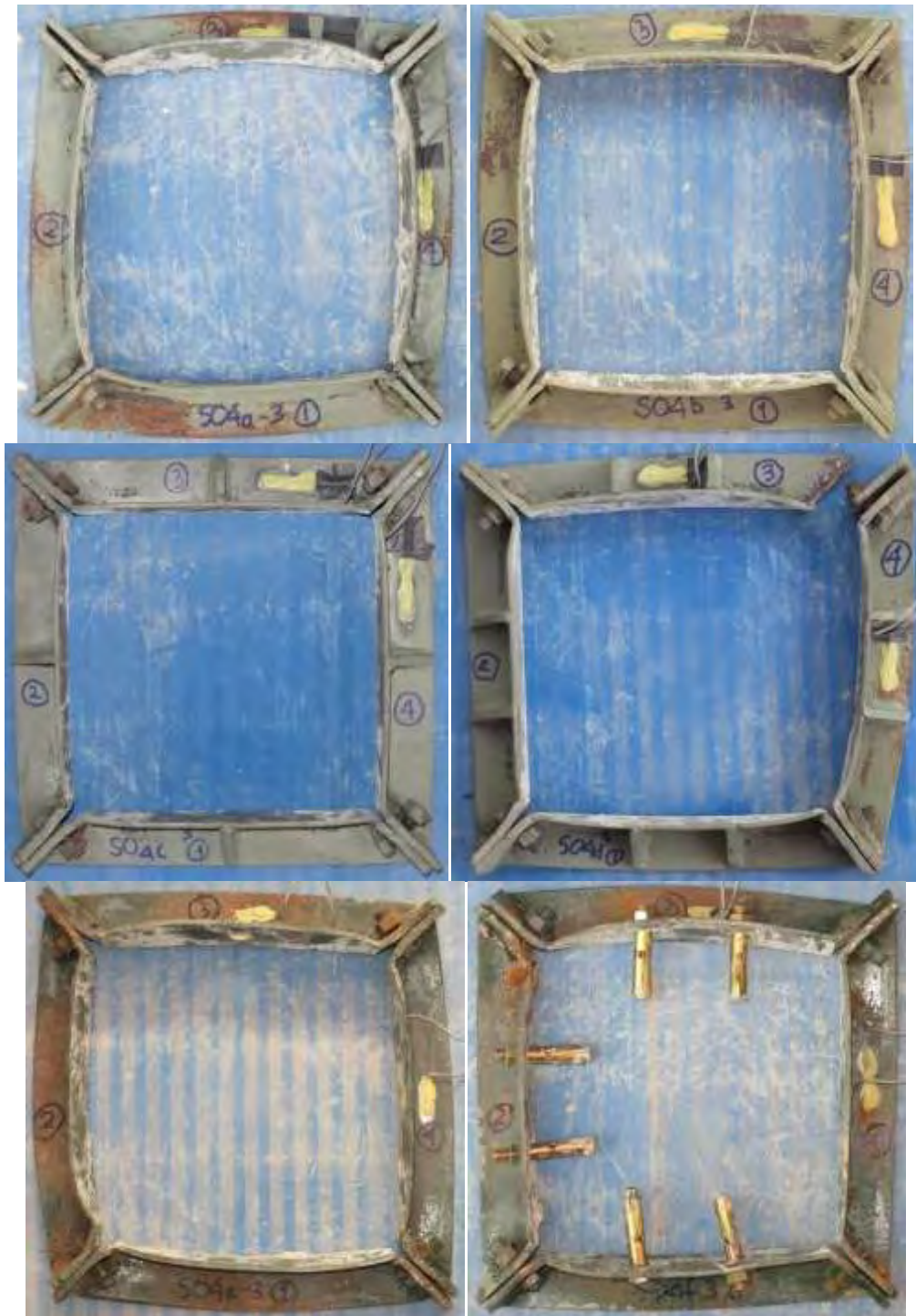
Figure 4-10 Steel collars of Specimens S04a, S04b, S04c, S04d, S04e, and S04f after completion of the tests
