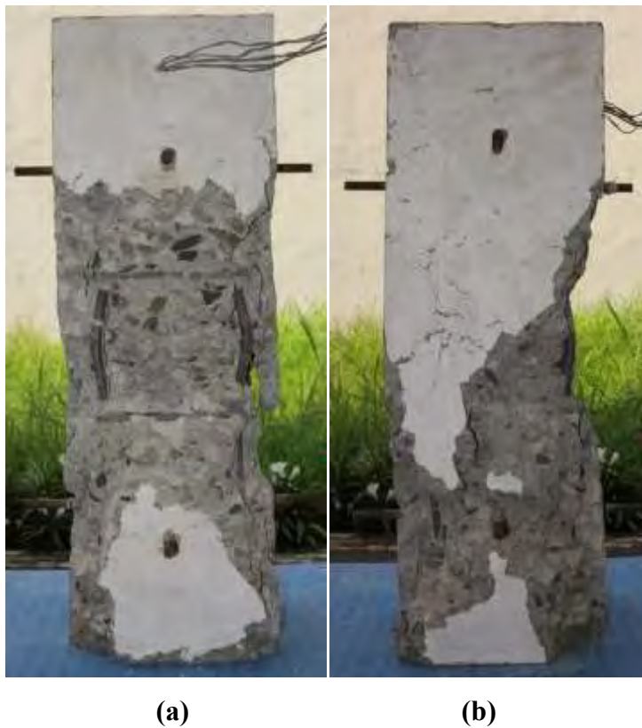
Figure B-8 Specimen CS02a: (a) side 1; and (b) side 2 after the completion of the test
