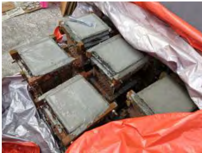
Figure 3-40 Cover of specimens to prevent direct sunlight
