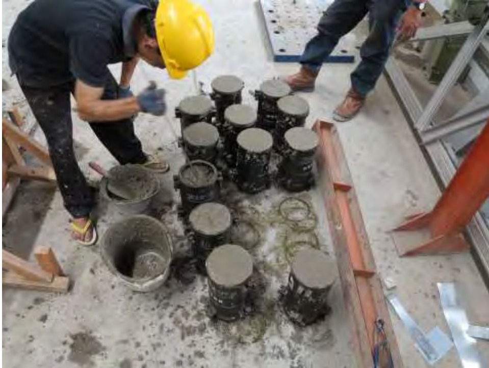
Figure 3-48 Concrete casting of standar cylinder
