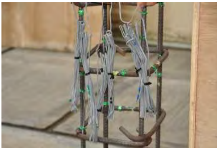
Figure 3-30 A sample of reinforcement cage with installed coded strain gauges (e.g. Specimen CS02a)
