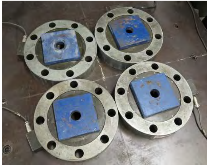
Figure 3-52 Four load cells with 50 ton capacity each
