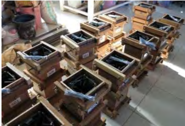
Figure 3-28 Formworks used for the specimens
