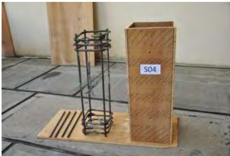
Figure 3-29 A sample of reinforcement cage (e.g. Specimen S04)
