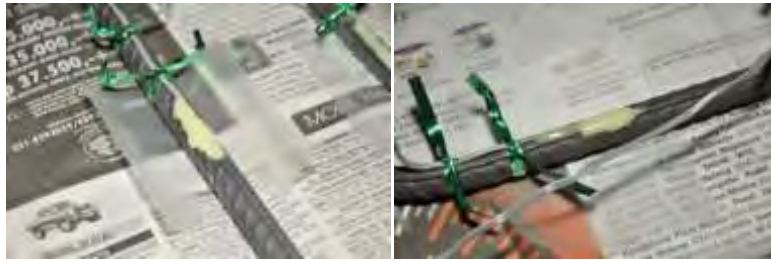
Figure 3-25 The strain gauges were protected by provided coating
