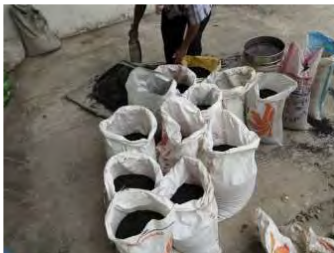
Figure 3-33 Lumajang sand used in the concrete mix
