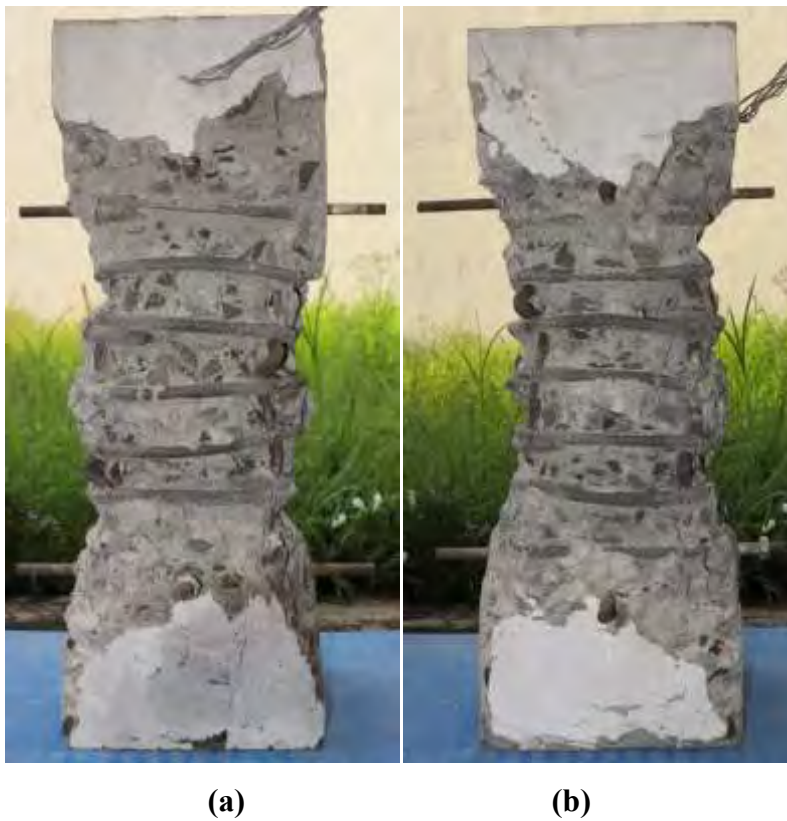
Figure B-12 Specimen CS03a: (a) side 1; and (b) side 2 after the completion of the test
