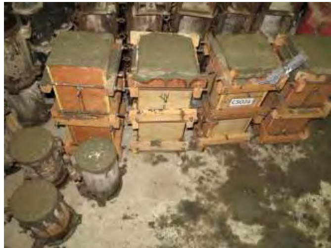
Figure 3-38 Molded specimens and standard cylinders
