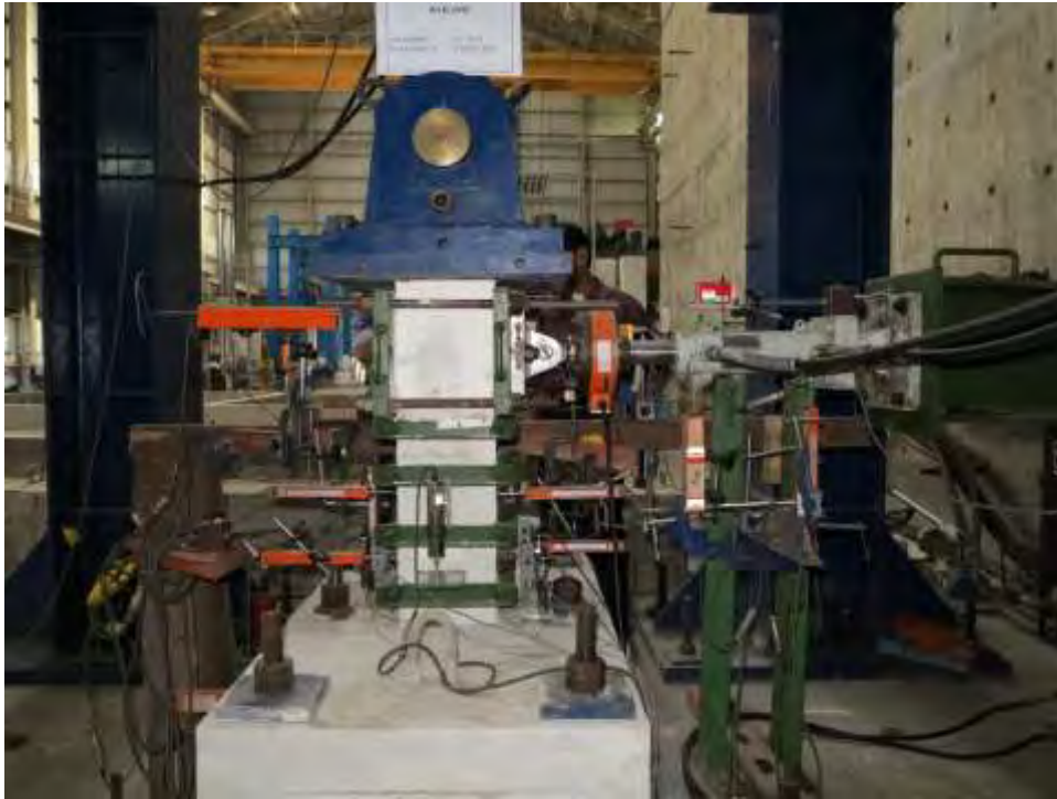
Figure 3-57 Typical setup for combined axial compressive and reversed cyclic lateral load test
