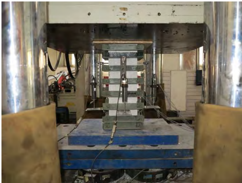
Figure 3-53 Typical axial compressive test set-up
