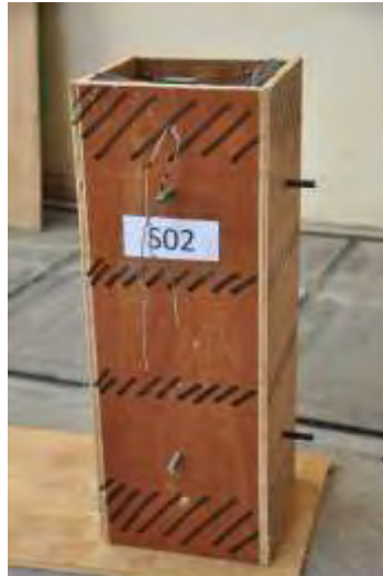
Figure 3-31 Typical rods installment for gauge length marking (e.g. Specimen S02)
