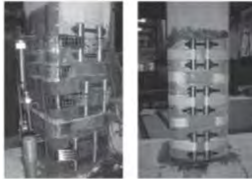
Figure 2-33 FRP jacketing method (courtesy of Nesheli et al., 2004)
