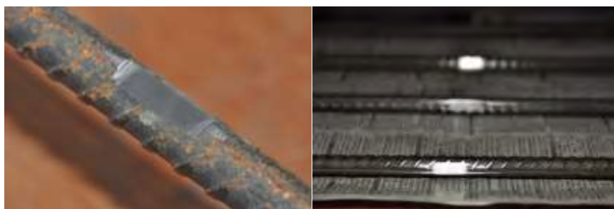
Figure 3-23 Flattened and smoothed surface of bars prior to the attachment of strain gauges
