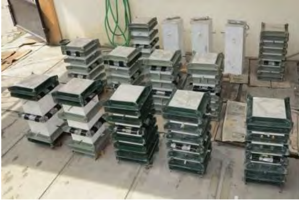
Figure 3-41 Externally collared column specimens
