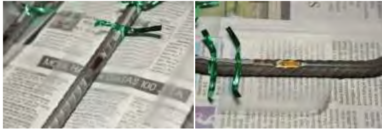
Figure 3-24 The strain gauges attached to the bars by using provided adhesive
