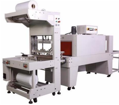
Figure 2. 3 Prometica Sleeve Wrapping Heat Sealing Machine
