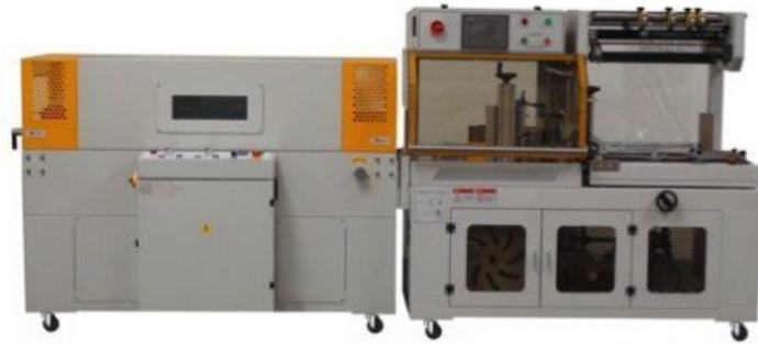
Figure 2. 1 EntrePack Automatic SW-1713 L-Bar Shrink Wrap Machine
