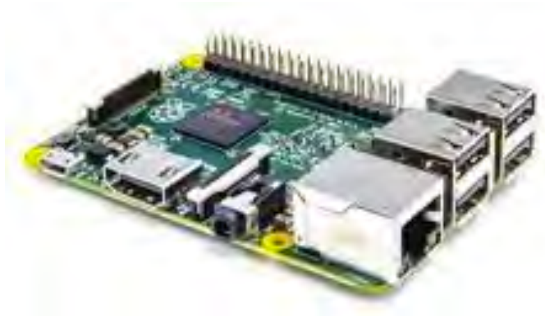
Gambar 2.5 Raspberry Pi 3 Model B
