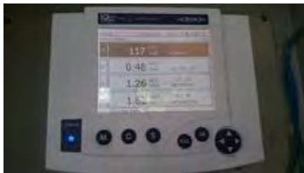
Fig. 3. WTW IQ SensorNet 2020 XT Controller
