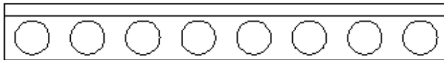
Gambar 2.1 Pelat pracetak berlubang ( Hollow Core Slab ) (Sumber: PCI Design Handbook 6 th Edition )
