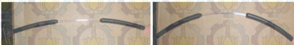
Gambar 2.6 (a) Probe sensor nafas, (b) Probe sensor pembanding
