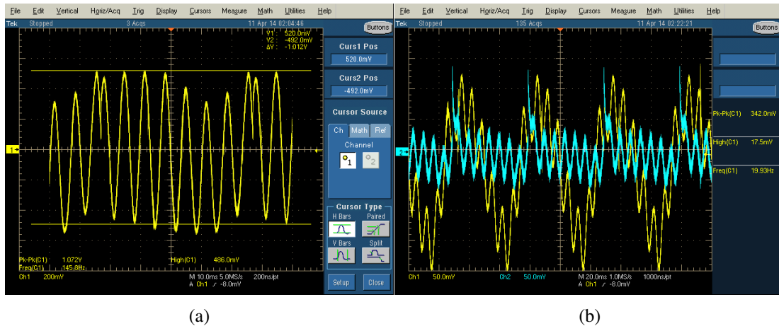
Figure 5.34: Loop test results with (a) 30 (b) 50 dB attenuator, the deramped frequency in both figures is 145 Hz, also note the 20 Hz PRF in (b)
