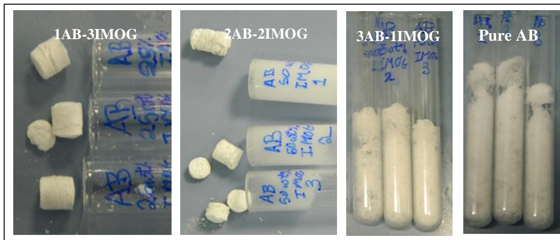
Figure 65: AB-IMOG pellets after foam testing.
