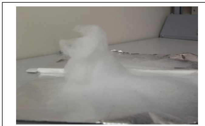
Figure 32: The fluffy fibres produced from the PEO-AB-ACN solution.
