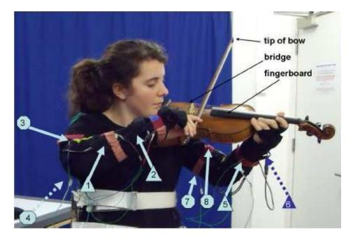
Figure A-7: First prototype (1 move bow hand forward, 2 move bow hand back, 3 move bow hand down, 4 move bow hand up, 5 move violin left, 6 move violin right, 7 move violin up, 8 move violin down)
