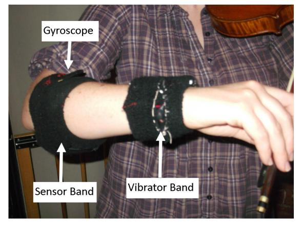
Figure 5-3: The sensor band worn on the forearm and the vibrotactile band worn on the wrist.
