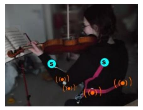
Figure 7-1: Photograph of the Buzzy Jacket. (S) Shows position of accelerometers. ((o)) Shows the position of the vibrators.
