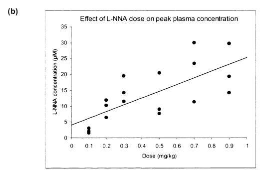
Figure 6.2 Relationship between N-nitro L-arginine (L-NNA) dose in mg/kg and L-NNA plasma area under the curve (AUC) (a), and peak concentration (b).
