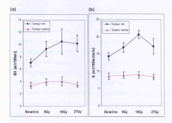
Figure 4.3 Line graphs showing mean changes (±1 standard error) in tumour blood volume (BV) (a) and transfer constant (K) (b) at the tumour rim and the tumour centre following fractionated radiation therapy. Increases in both vascular parameters were greater at the tumour rim compared to the tumour centre.
