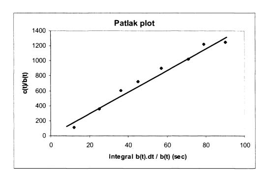
Figure 2.5 Patlak plot is shown for a study patient. The transfer constant K is derived from the gradient of the line, and relative blood volume (BV) from the y-intercept.
