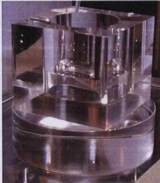
**Figure 2.6:** Perspex mimic of a single well for a 24-SRW (ULA) plate used for mixing time studies. Dimensions of the well were the same as the actual wells from the microplate. The faces were square to avoid image distortion during high-speed video footage.
