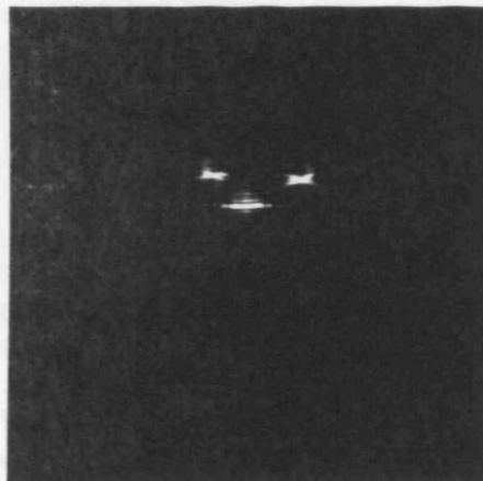
Figure 2.13: ISAR image of three metal-spheres: L \times W = 3.024\text{ m} \times 1.185\text{ m} , \Delta r = \Delta r_c = 24\text{ mm}
