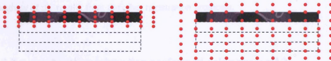
Figure 4.1 - Illustration of Control Point (CP) placement in the standard (left) and extended (right) CP grids. The Cine CT volume being registered (from the most Superior couch position) is shown, the dashed lines indicate the other three couch positions where data has been acquired, and the CP positions are shown in red. It can be seen that the standard CP grid only covers the image being registered (plus one CP outside so that the deformation is defined over the whole image), whereas the extended CP grid covers all of the couch positions where data has been acquired.
