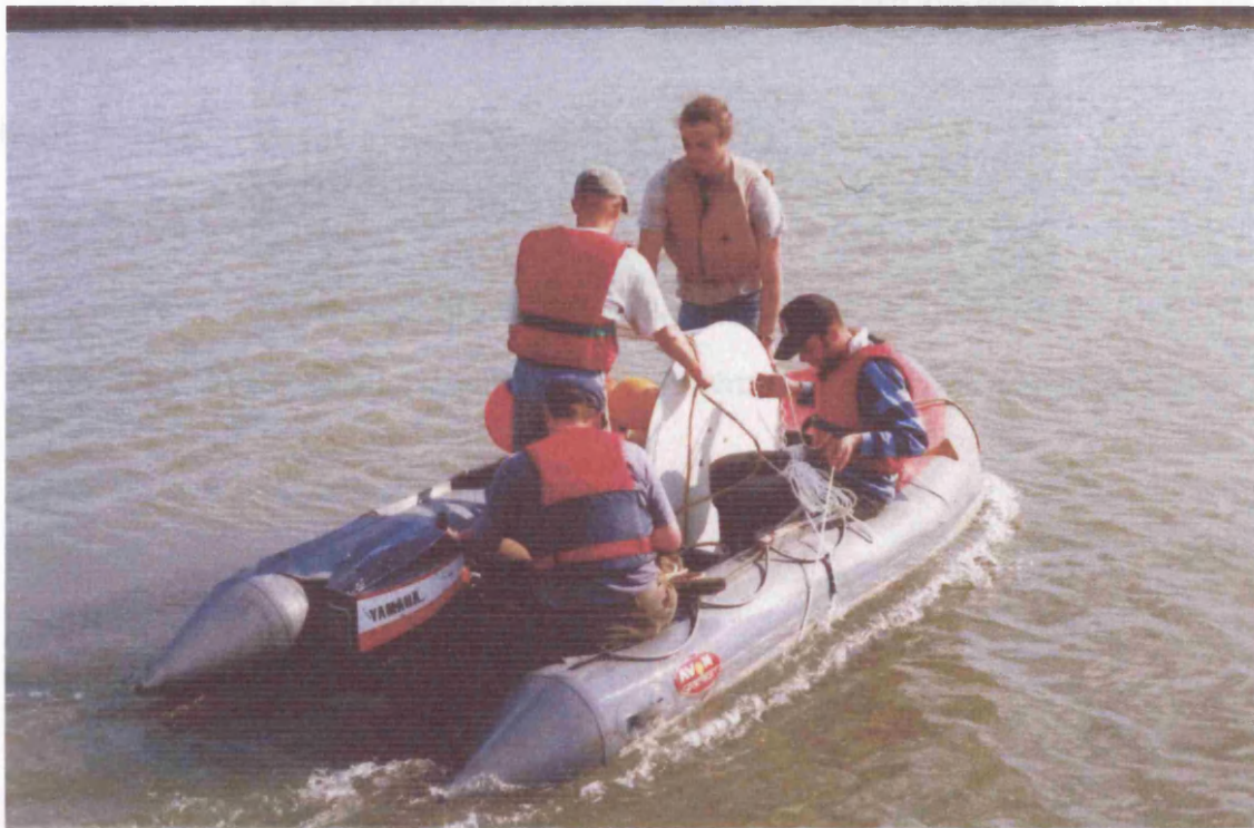
Figure 2.6 – Deploying the ADCP bottom rig at Reydon.
