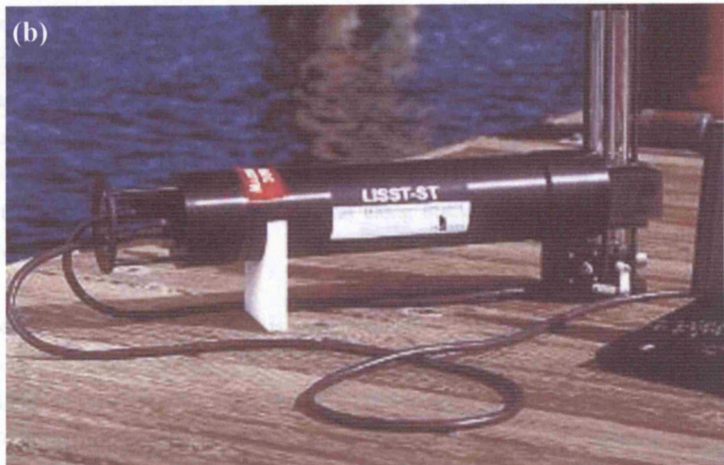
Figure 3.5 – Field deployable laser diffractometers. (a) The adapted Malvern particle sizer used by Bale & Morris (1987): (i) Fourier Transform lens, (ii) detector, (iii) He/Ne laser, (iv) light guide, (v) sample volume. (b) LISST-ST with automated settling column (from Sequoia Scientific Inc.; http://www.sequoiasci.com ).
