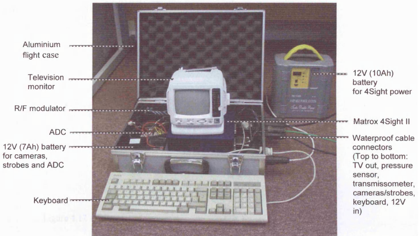
Figure 4.11 – Customised housing for computer components
