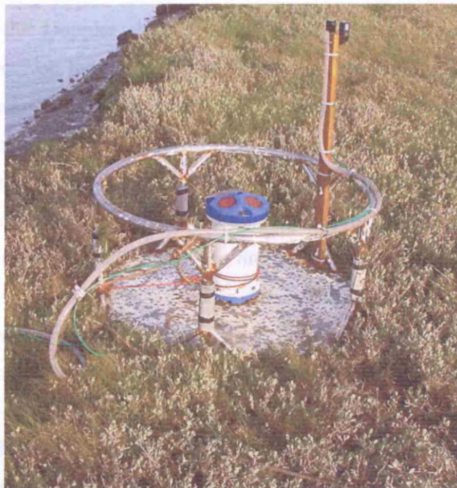
Figure 1.10 – Photo of RD Instruments Workhorse broadband ADCP on customised mount (with Partech IR40 transmissometer and pump sampler intake tube on a 1m pole) prior to field deployment.
