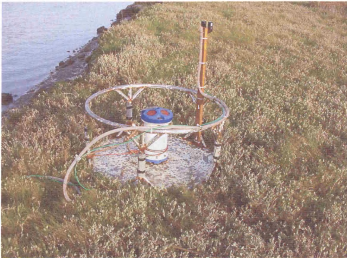
Figure 2.5 – The ADCP bottom rig (with transmissometer and water sample hose)
