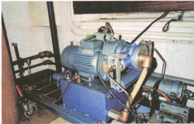
2) Above: Confining pump
