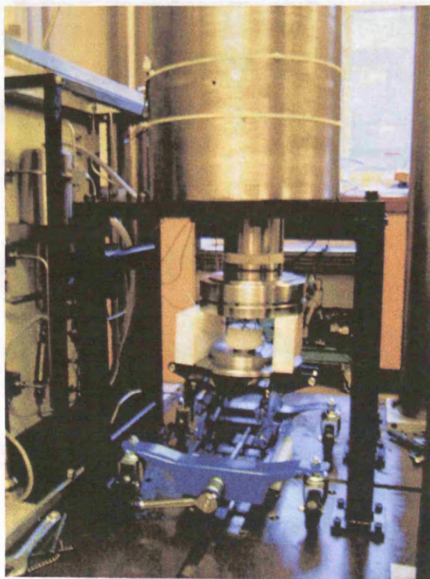
1) Above: Putting the furnace into the pressure vessel using the jack and support frame
