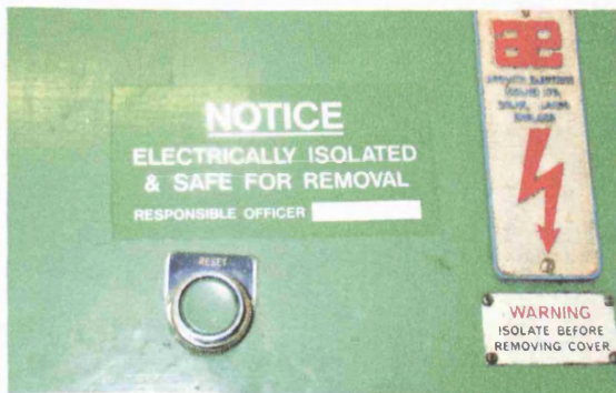
2) Above: Emergency reset button located on the back of the coring machine
