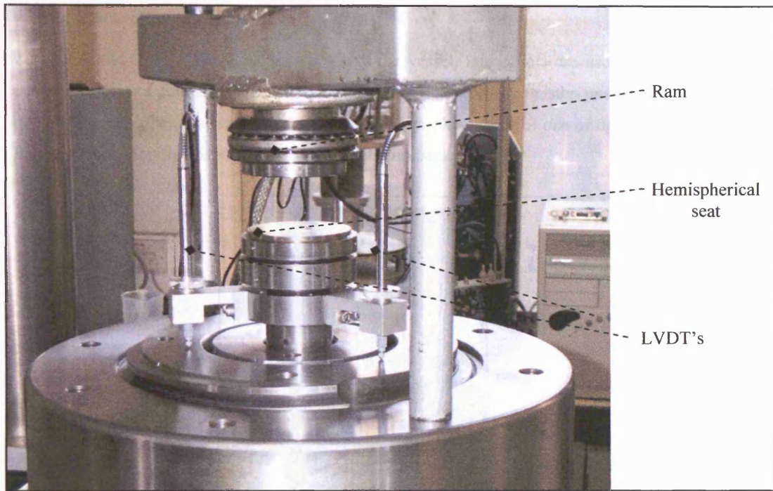
Figure 4.4: Photograph of LVDT's attached to top of the pressure vessel.
