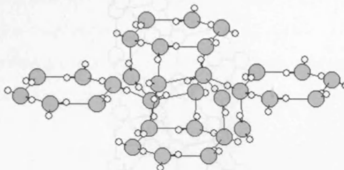
Figure 2.6: The ice II structure in [001] projection. Large grey spheres show oxygen positions, while the smaller white ones are the hydrogen positions.
