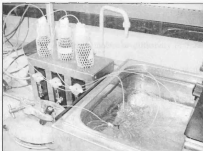
Figure 4.2: Experimental setup for continuous epoxidation experiments
