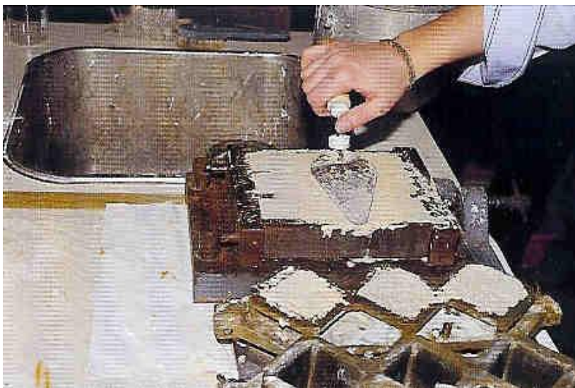
Figure 84: laboratory experiment for production of artificial stone (source: Makryodi et al. 1999, 88).
