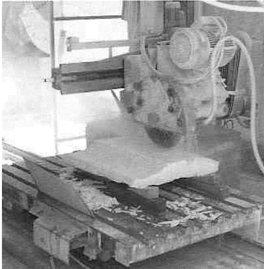
Figure 52a: the marble cutter of the Parthenon work-site (photo by Maurommatis, 2002) (source: SRAM 2002, 9).
