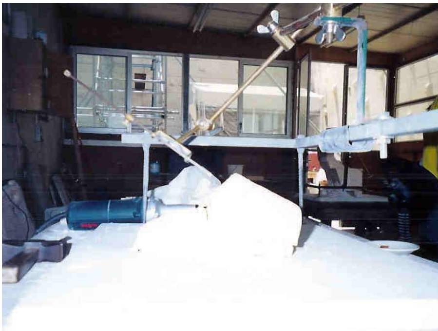
Figure 52d: pantograph used for producing new members and additions in the restorations of the Acropolis monuments (source: Vacharopoulou -- personal photographs, 2002).
