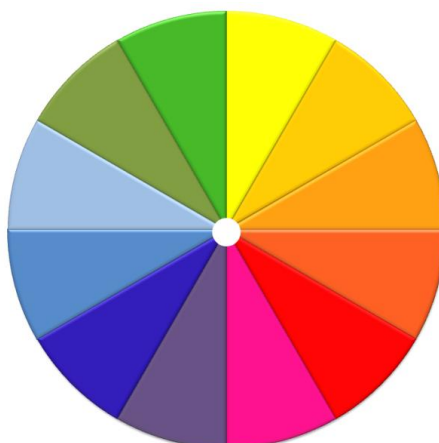
Figure 5.02: Prediction of the absorbed wavelength according to observed colours by the use of the colour wheel. The colour wheel is an abstract illustration of the circular organisation of the colour hues. It is used for the ascertainment of the complementary colours, which lay in opposition to each other in the wheel. According to the oxford dictionary a complementary colour is “a colour that combined with a given colour makes white or black”. Complementary colours are the link between the observed colour and the prediction of absorbed wavelength for a coloured compound of interest.
