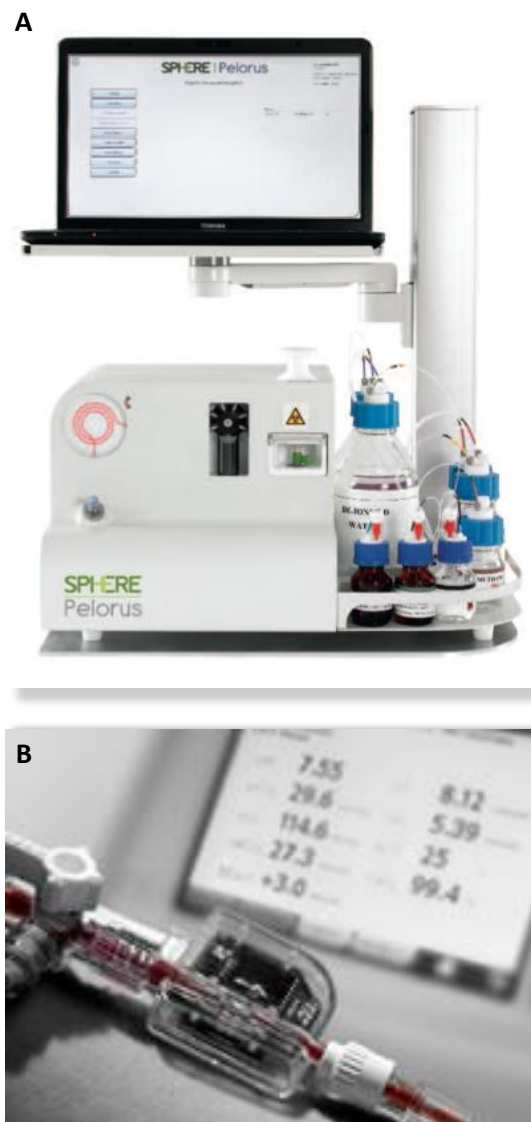
Figure 4.02: Point-of-care sensors developed by our Industrial Partner – Sphere Medical Ltd., Cambridge. A) Pelorus propofol measurement system. It measures rapidly the concentration of the intravenous anaesthetic propofol in whole blood samples and therefore enables an optimal therapy at the individual patient level. Image adopted from “Sphere Medical Ltd.’s Homepage: Pelorus Propofol Measurement System” 2014. B) Proxima system. It is a disposable multi-parameter micronalyser of arterial blood, which is patient attached and measures the blood gases, haematocrit and electrolytes on demand in real-time. Image adopted from “Sphere Medical Ltd.’s Homepage: Proxima System” 2014.
