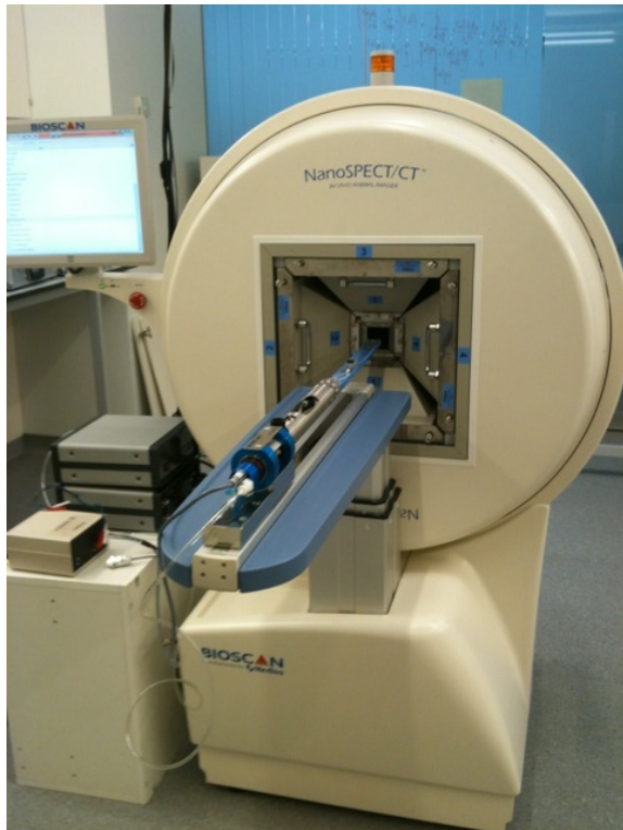
Figure 2.3: The NanoSPECT/CT system used for imaging, with physiological monitoring systems for in vivo imaging.
