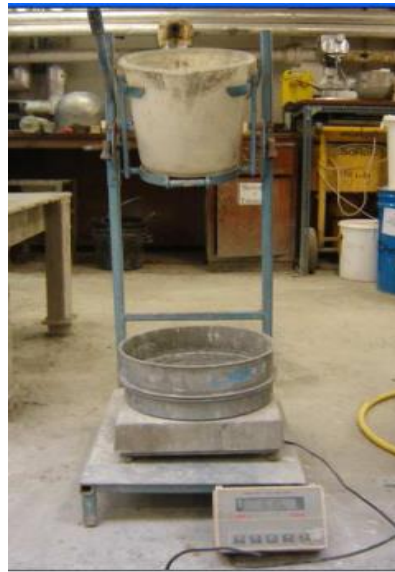
Figure 4-11 Sieve segregation test apparatus for SCC
