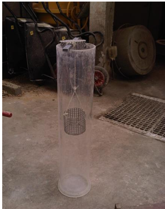
Figure 4-13 Plunge test apparatus for UWC
