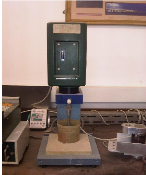
Figure 4-5 Rheomat Rheometer 115 apparatus
