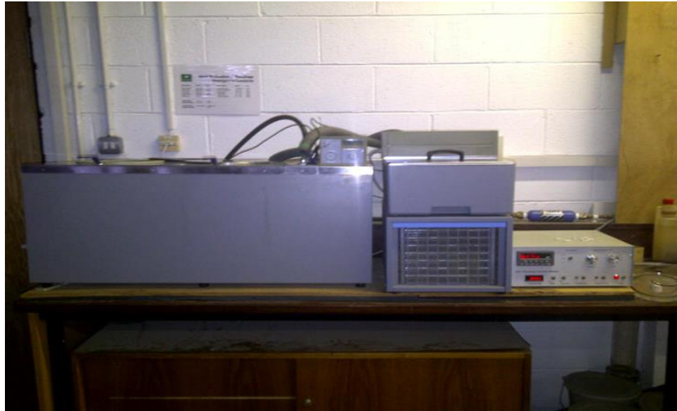
Figure 4-1 JAF isothermal conduction calorimeter set-up
