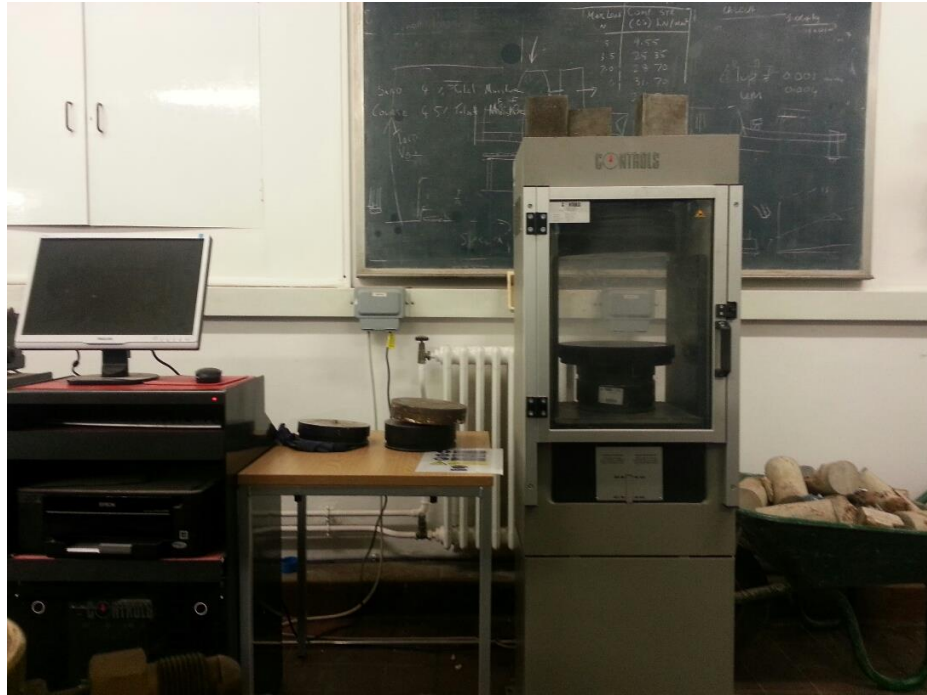
Figure 4-14 Uniaxial compression test machine
