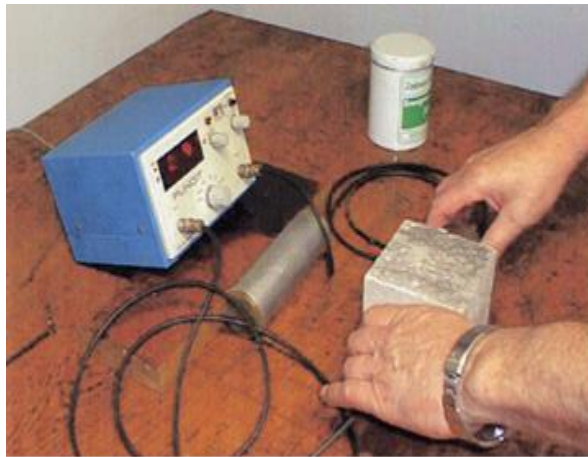
Figure 4-15 The Pundit apparatus
