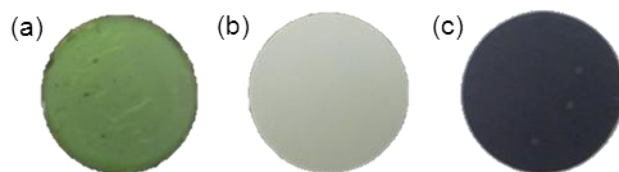
Figure 4-8: SOEC cells after sintering; (a) Ni-CGO cathode, (b) YSZ electrolyte, (c) LSM anode.
