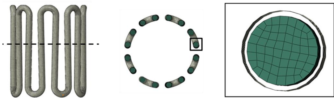
Figure 5.10 - Stent crown surrounded by a shell, created as a 0.02 mm offset from the external elements of the stent crown.
