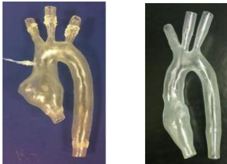
Figure 6.1 - Rapid prototyped rigid 3D models of the aortic arch of the TGA (left) and the Control (right) patients.
