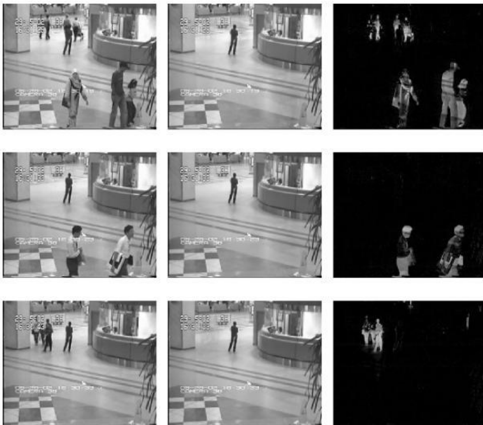
Figure 4.3: Application of RPCA to background modelling in video surveillance data (images taken from [102]).
