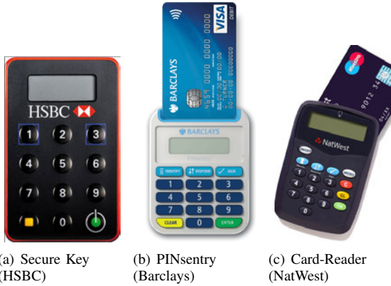
Fig. 1: Examples of three hardware tokens, i.e., devices generating one-time passwords (OTPs) for authentication purposes.
