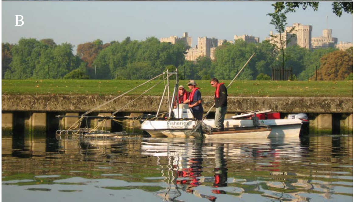
Figure 3.4 Typical electrofishing procedure carried out by the Environment Agency, to obtain roach samples. Two methods are commonly employed where (A) in shallow waters, fish can be stunned using two hand-held anodes powered by a battery and transformer contained in the boat. Fish swim towards the anode, are stunned, and then caught in a net. In deeper water, (B) electrofishing is conducted using a 'boom boat'. The boat itself is the cathode, and the anodes are mounted off the bow. The stunned fish swim toward the anode, where they are then caught using a dip net
