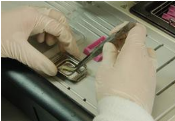
Figure 5.5 (A) Typical procedure of placing processed tissue into a mould filled with wax, obtaining the correct orientation for subsequent sectioning. Once the cassette case has been replaced on top of the sample, refilled with wax, and then cooled, it can be removed from the mould (B) and be ready for sectioning on a microtome
