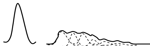
Figure 5 Temporal intensity profile of the laser before and after pulse stretch.
