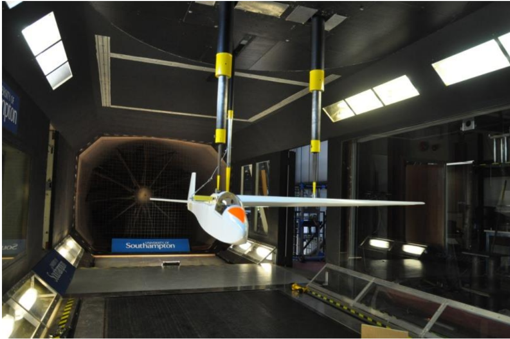
Fig. 2: A model of the 1:4 T.45 glider in the R.J. Mitchell wind tunnel (Photo: University of Southampton)
