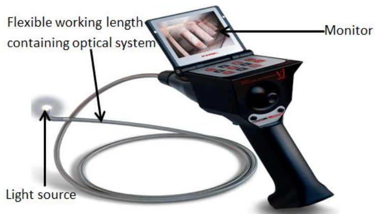
Fig.1.9: Advanced video borescope used for remote visual inspection [70].
