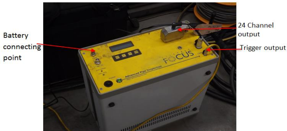
Fig.5.31: Pictorial representation of the teletest focus mark III pulser/receiver system showing the 24 channel output and the trigger output to the vibrometer unit [32].
