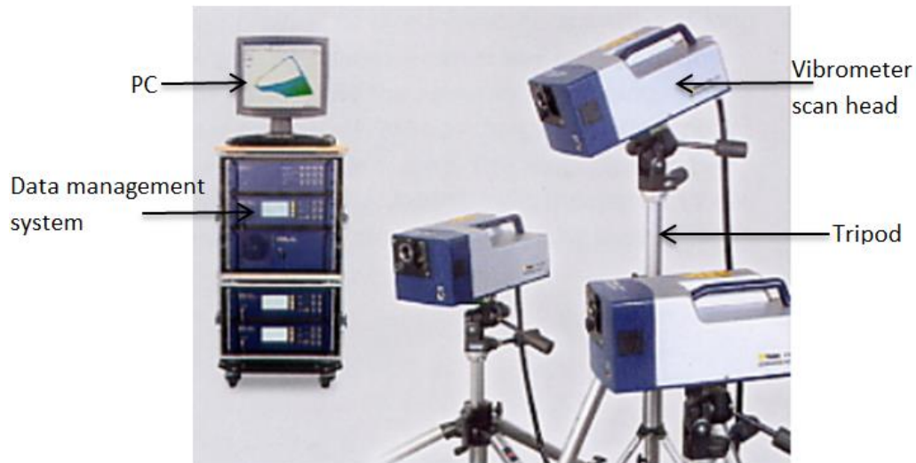
Fig.5.32: Pictorial representation of the PSV-400-3D scanning vibrometer used in the model validation experiment [176].
