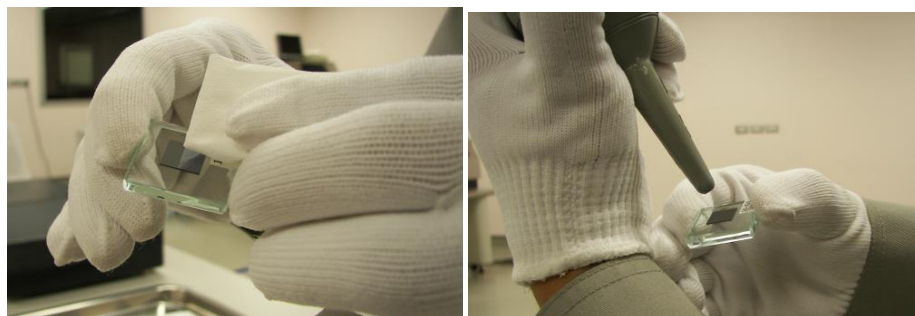
Figure 4.3 Cleaning process (wiping – left and blow drying – right).
