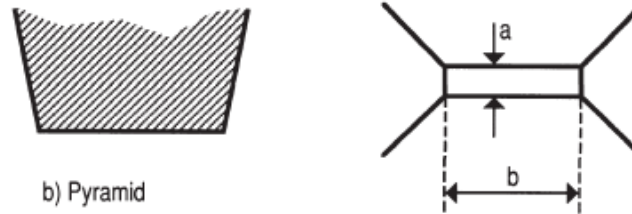
Figure 2.3 Pyramid-shaped stylus (geometry shown to the right). Image reproduced from (Whitehouse, 2000).
