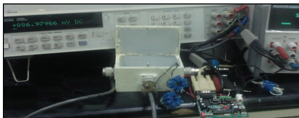
Figure 2. Automated system of the multiple output \mu pot.
