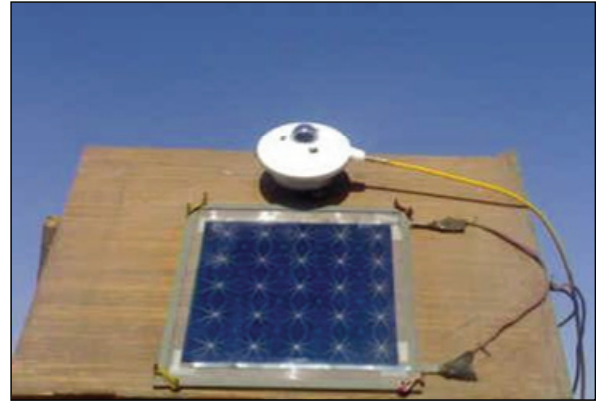
Figure 1. Multicrystalline silicon solar cell in the outdoor located at optimum tilt angle with the radiation sensor.
