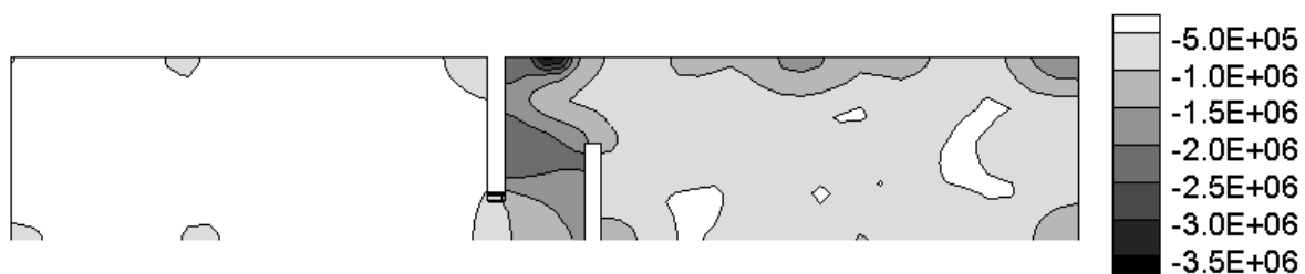
Figure 2. Predicted minimum acoustic pressure (Pa) in domain for a configuration with baffles separated at a distance of 0.5 \lambda for water.
