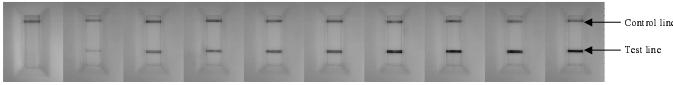
Fig. 2. Images of gold immunochromatographic strip of different concentration (from the left side: 0, 10, 35, 75, 100, 150, 200, 300, 400, 500mIU/ml).
