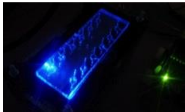
Fig. 7. PDMS glass microfluidic device for 6-plex amplification and detection
