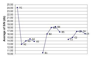
**Fig. 3.** Influence of design parameters on *S/N* ratio for a set of 25 models defined by the OA  $L_{25}$  (Table 2).
