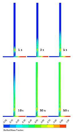
**Fig. 4.** Mass fraction contours on a mid-height plane at different times of design case 3 of Table 2 (f = 1 Hz,  $\phi = \pi/2$ ,  $\theta = 180^{\circ}$ ), showing only 5 mm of mixing channel length.
