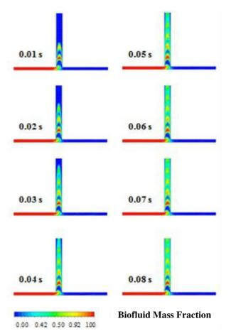
**Fig. 8.** Mass fraction contours on a mid-height plane at different times (case: f = 100 Hz,  $\phi = \pi$ ,  $\theta = 180^{\circ}$ ) ), showing only 1.3 mm of mixing channel length.
