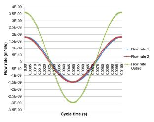
**Fig. 10.** Flow rate in the inlet and mixing channels of the micromixer in a representative work cycle of design case 21 of Table 2 (f = 100 Hz,  $\phi = \pi/36$ ,  $\theta = 240^{\circ}$ ).
