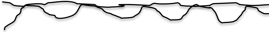
(a) For the rough surface ( R_a : over 0.01); the rate of surface contacts is high
