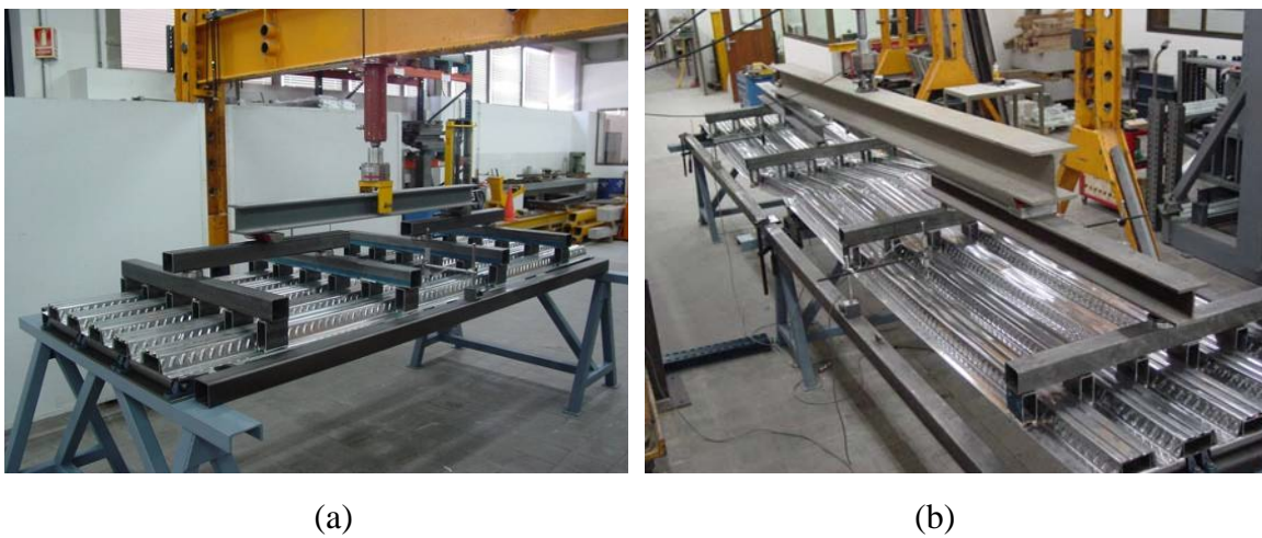
Figure 8 (a) Simply supported decking tests and (b) Continuous decking tests [17]
