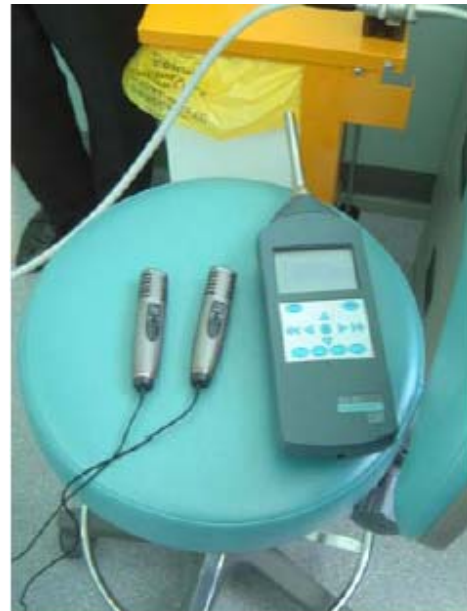
Figure 6: Cel analyser and Sony microphones used.
