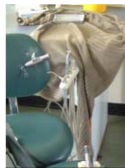
Figure 2 Free running test in dental clinic This gave repeatable measurements with an average dBA reading for successive tests on the same handpiece with the
