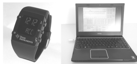
Fig. 1 Wireless watch eZ430-Chronos with a mobile computer
