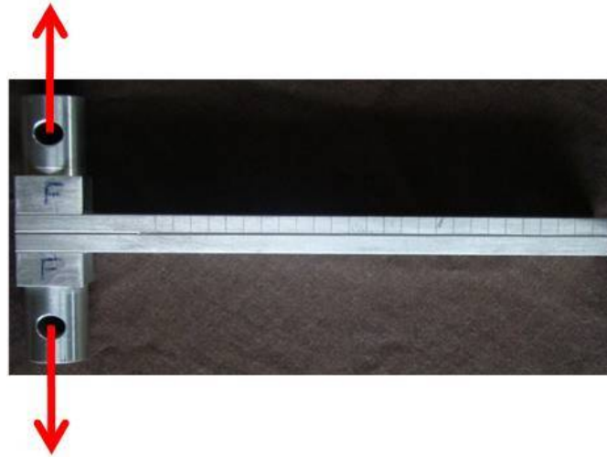
Figure 6: DCB adhesive joint tested [30].
