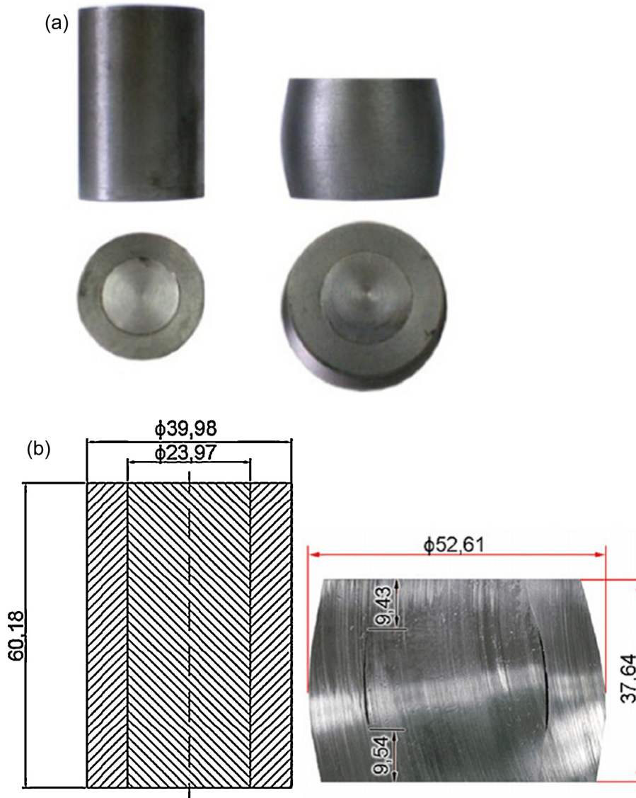
Fig. 4. Initial and compressed billet (a) initial and compressed bi-metal ring and (b) meridian cross section of bi-metal ring after compressed ( Essa et al., 2012 ).
