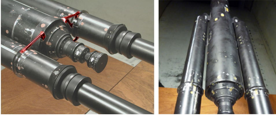
Fig. 2. Ariane 5 launcher model in the NLR wind tunnel. Left-hand side: Configuration A . Right-hand side: Configuration B . (For interpretation of the references to color in this figure, the reader is referred to the web version of this article.)
