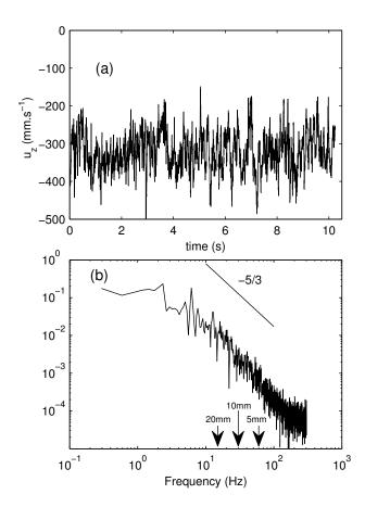
FIG. 6. Velocity measurements for a flow rate of  $0.62 \text{L·s}^{-1}$  and a rotation rate of 1.5Hz. (a): time signal of the vertical velocity  $u_z$  at point x = -0.3, y = 0, z = -140 (in mm). (b): corresponding power spectrum. Arrows stand for corresponding length scales using Taylor's hypothesis.
