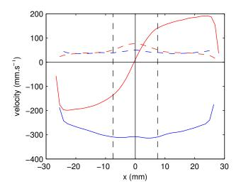
FIG. 4. Velocity profiles at  $z=-140 \mathrm{mm}$  along x-axis, for a flow rate of  $0.62 \mathrm{L \cdot s^{-1}}$  and a rotation rate of 1.5Hz. Blue: vertical velocity  $u_z$  (solid line) and its standard deviation  $\sigma_{u_z}$  (dashed line). Red: tangential velocity  $u_y$  (solid line) and its standard deviation  $\sigma_{u_y}$  (dashed line). The vertical dashed lines stand for the core region of diameter 15mm.
