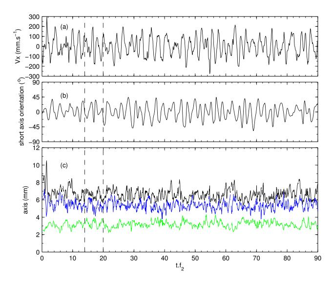
FIG. 9. Time signals of (a): horizontal velocity  $V_x$ , (b): orientation  $\theta$  of the short axis relative to vertical direction, and (c): semi-axis lengths (black: a, blue: b, green: c) for sequence B5. All the times are made non-dimensional with  $f_2 \simeq 15$ Hz. The vertical dashed lines stand for the time interval corresponding to the sequence depicted in Fig. 8.
