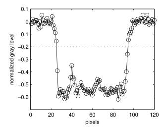
FIG. 2. Normalized gray level profile along constant height  $z=-146.5 \mathrm{mm}$  for view 1 of image 39 of sequence B5 (see also top left quadrant in Fig. 3). Horizontal dotted line: threshold used for binarization. Bubble corresponds to values below the threshold. Calibration factor: 6.5 pixels corresponds to 1mm.
