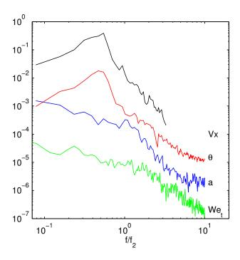
FIG. 10. Power spectra of (black):  $V_x$ , (red):  $\theta$ , (blue): a for sequence B5 (please see also the time signals in Fig. 9) and (green):  $We_t$  at point x=-0.3, y=0, z=-140mm (please see the time signal in Fig. 7). The frequencies are made non-dimensional with  $f_2 \simeq 15$ Hz. The different spectra have been vertically shifted for the sake of clarity.
