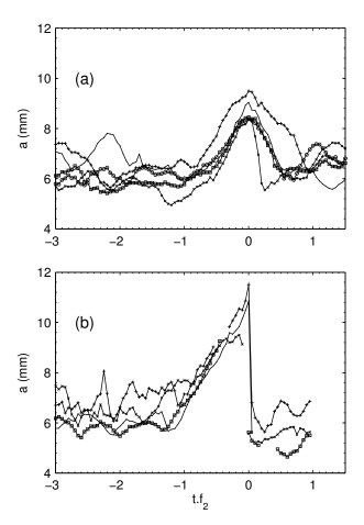
FIG. 13. Superposition of large deformation phases (a) and breakup events (b) for the different bubbles. The sequences have been synchronized on the maximum of a. The time is made non-dimensional with  $f_2 \simeq 15$ Hz. (a): case B2 ( $\square$  and  $\circ$ ), case B3 ( $\times$ ), case B4 (black line) and case B6 (+). (b): case B2 ( $\square$ ), case B3 ( $\times$ ), case B4 (black line) and case B6 (+).
