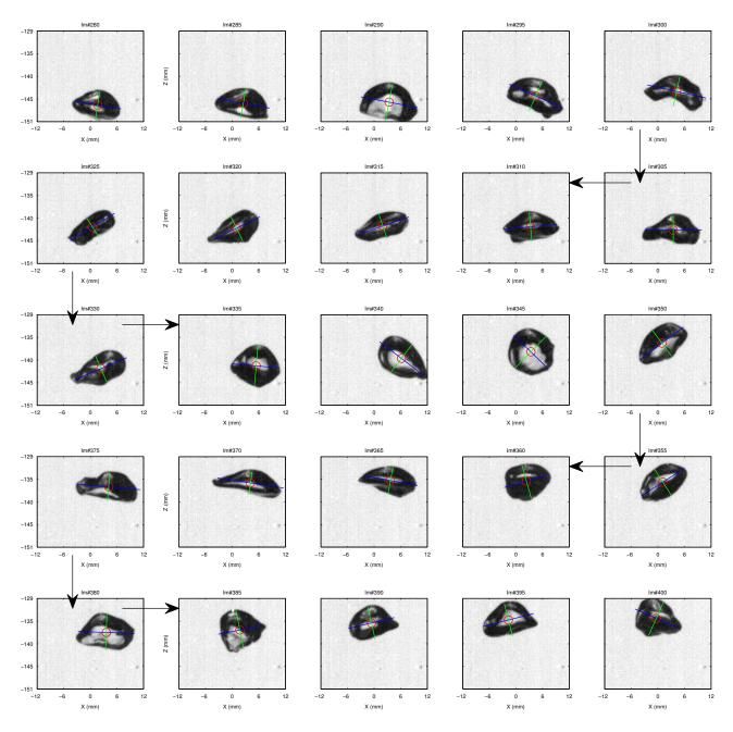
FIG. 8. Illustration of a deformation sequence on case B5. Side view in the plane x-z (camera 1) with the center of mass (red dot), the major (blue line) and minor axes (green line) of the equivalent ellipse. One image over 5 is displayed and the time lag between each image thus corresponds to 1/60s ( $(4f_2)^{-1}$ ). Please note that the sequence reads from top left to top right then the second line reads from right to left, and so on, following the arrows.
