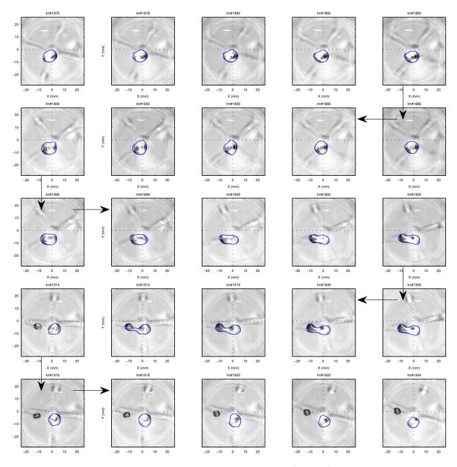
FIG. 15. Illustration of a breakup on case B2. Bottom view in the plane x-y (camera 2) with the detected contour in blue. One image over 2 is displayed and the time lag between each image thus corresponds to 1/150s ( $(10f_2)^{-1}$ ). Please note that the sequence reads from top left to top right then the second line reads from right to left, and so on, following the arrows.
