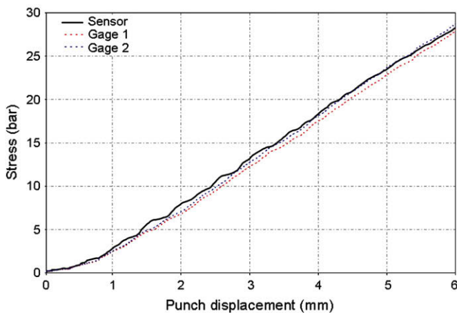
Fig. 7. Pressure (measured by piezoelectric sensor and obtained by gages) in the hydrostatic chamber as a function of punch displacement of the flywheel. This dynamic test was done with a rigid metallic sample.
