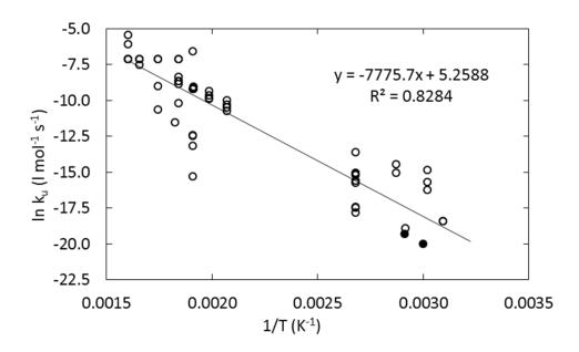
Figure 5. Arrhenius plot of  $k_u$  values from literature ( $\circ$ ) and obtained in this work ( $\bullet$ ).
