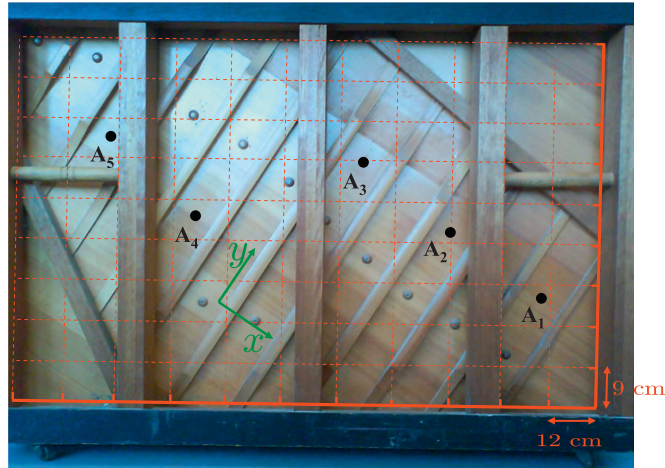
Fig. 7. Rear view of the upright piano, with the mesh for modal analysis (in red) and the locations of the five accelerometers (in black). (For interpretation of the references to color in this figure caption, the reader is referred to the web version of this article.)
